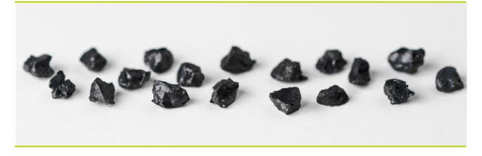
NAstra® is a decorative mineral building material based on iron silicate in accordance with EN 12620.
